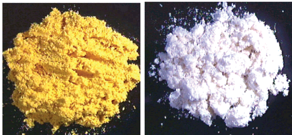
Figure 7. View of a sample of poly[diaqua- (\mu_2 -squatato- O,O' )- (\mu_2 -4,4'-bipyridine- N,N' )-manganese(II)] trihydrate in which the water was completely removed (left) and after it was stored in a saturated air atmosphere (right).
